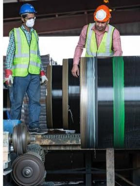
Application of External CWC: Concrete Weight Coating to Double Joint Welded (24 Meters) Pipes Concrete Weight Coating Thickness Range: From 1" to 6"
